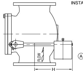
NOTE: SUFFIX "A" USED AFTER FIGURE NUMBER FOR VERTICAL INSTALLATION (FIG.NO.220-DA)
