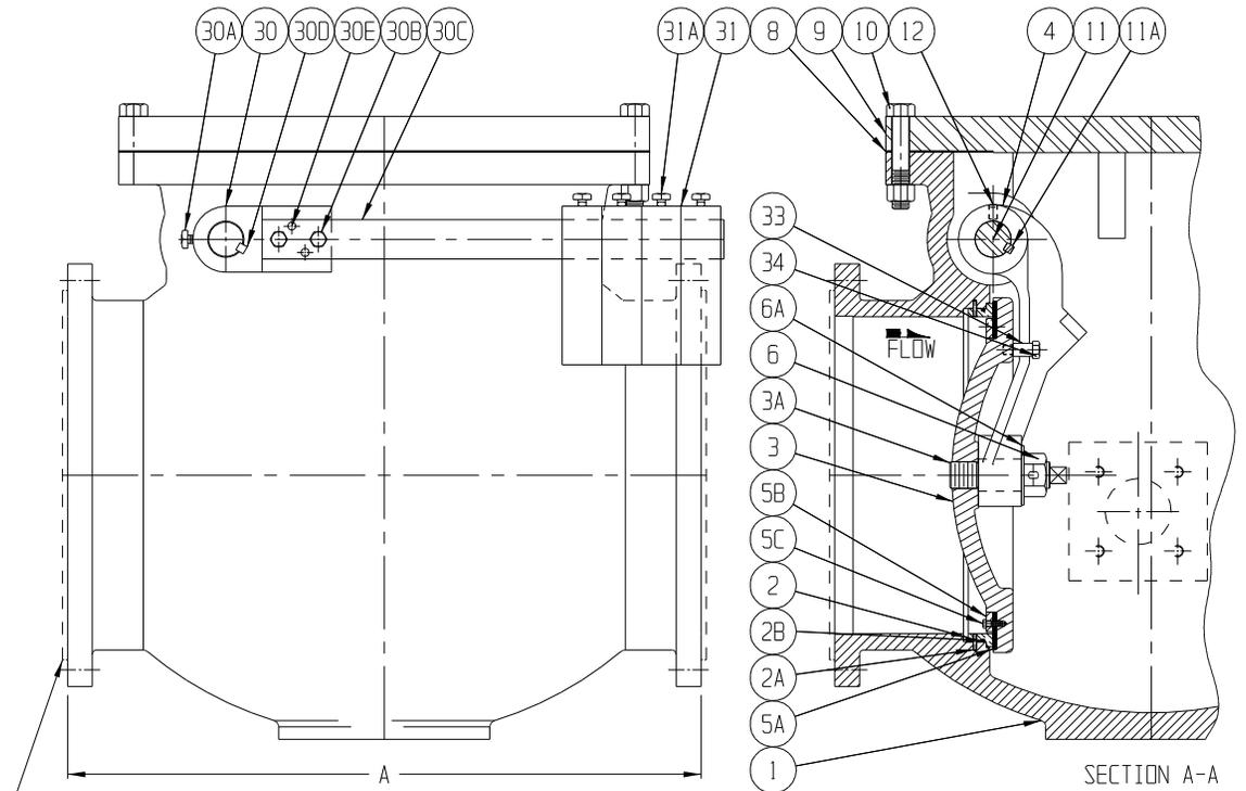
NOTE: "A" DIMENSION ON VALVES WITH RAISED FACE FLANGES DOES NOT INCLUDE THE RAISED FACE HEIGHT
