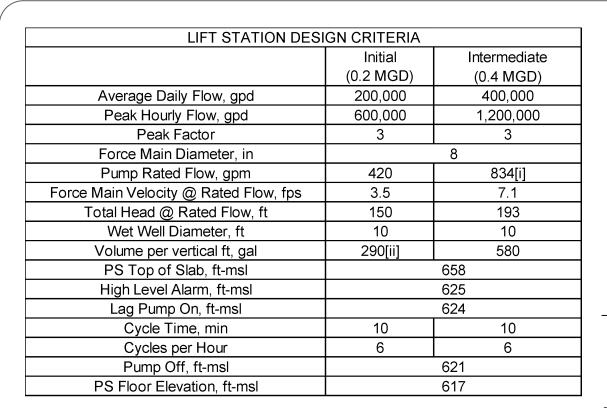
[i] 2-pump operation [ii] With vertical partition, only half of wet well utilized in early stage
